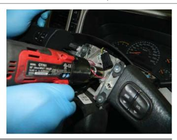
**STEP 9:** Reconnect airbag assembly electrical connectors.
