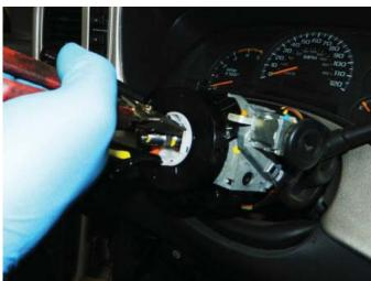
**STEP 7:** Remove the orange stop clip from the clock spring.
