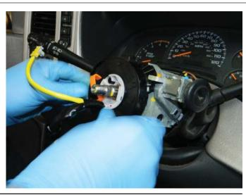
**STEP 6:** Using pliers, reinstall clock spring retaining ring.
