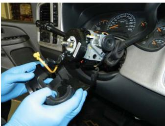
**STEP 11:** Using pliers or picks, remove the clock spring retaining ring.
