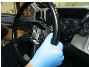
**STEP 9:** Using a flat-blade screwdriver, pick, or other non-marring tool, release the upper and lower steering column covers.
