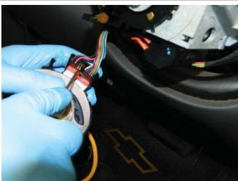
**STEP 17:** Carefully peel the ribbon connector from each wire bundle.
