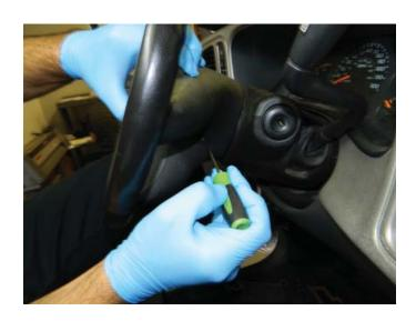
STEP 5: Remove steering wheel airbag.
