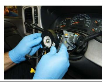
**STEP 13:** Position wire connector bundles and install wire segregator clip 1/2" from clock spring as shown. **Warning!** Failure to install connectors in the correct orientation could result in malfunction of the airbag system or inadvertent airbag deployment causing injury or death.
