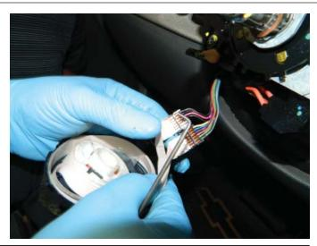
**STEP 16:** Using a small flat-blade screwdriver or pick, remove the orange bands from each of the wire bundles.
